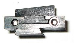
The amount of lead may be regulated by turning the respective stop screws in the side with the Allen wrench provided. Turn clockwise if you need less lead; turn counter-clockwise if you need more lead. The left screw is for the left-to-right lead, the right screw is for the right-to-left lead. The screws are retained with blue Loctite, so they are adjustable, but will stay where you turn them to.
